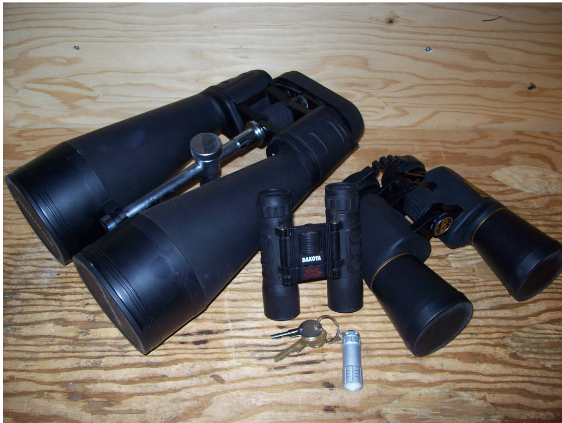
DISPLAY OF BINOCULARS. The smallest pair of binoculars here won't let in enough light for stargazers. The big set weighs 10 pounds. That's just too heavy to hold. The mid-size models are just the right compromise at 7 × 50.
